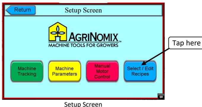
10. Tap “Select/Edit Recipes” to access “Recipe Setup” screen. **Note:** if the machine is integrated into a recipe soil system, this will be disabled. Skip to 14. and continue with remaining settings.
