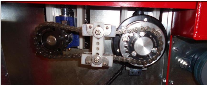
Regularly inspect the infeed drive chain. A damaged or loose drive chain can cause an improper soil mix. If the chain is found to be damaged, loose, or malfunctioning, repair immediately. Contact the manufacturer for the replacement parts.
