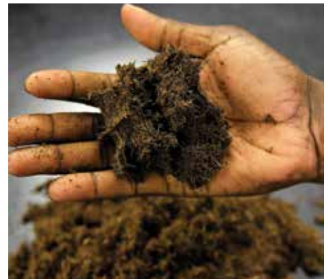
OPTIMAL MIX MOISTURE: SOIL BALL HOLDS ITS FORM SOMEWHAT, YET SLOWLY EXPANDS
