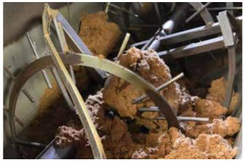
The numbers noted in the scenario below are based on using a Ribbon Blender that holds 3 cu. yds. to make a 60% peat: 40% HydraFiber EZ Blend mix. The HydraFiber technical team can provide adjustments to fit your specific blending formulation and equipment size.
