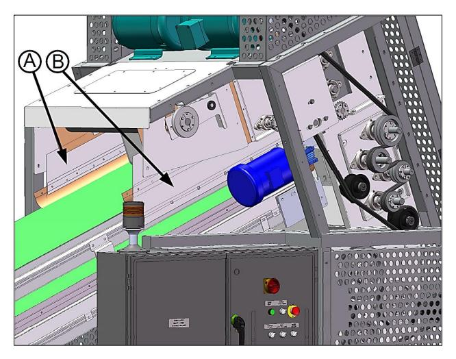
1) Utilizing hardware and square nuts allocated in upper conveyor, install bale guide panels (panels A and B).
